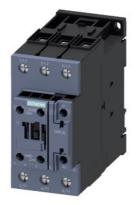
power contactor, AC-3e/AC-3, 41 A, 18.5 kW / 400 V, 3-pole, 175-280 V AC/DC, 50/60 Hz, with integrated varistor, auxiliary contacts: 1 NO + 1 NC, screw terminal, size: S2
