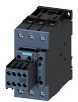
power contactor, AC-3e/AC-3, 41 A, 18.5 kW / 400 V, 3-pole, 24 V DC, 0.8-1.2\* Us, with integrated varistor, auxiliary contacts: 2 NO + 2 NC, screw terminal, size: S2, suitable for PLC outputs, removable auxiliary switch
