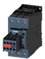
power contactor, AC-3e/AC-3, 41 A, 18.5 kW / 400 V, 3-pole, 24 V DC, 0.8-1.2\* Us, with integrated varistor, auxiliary contacts: 2 NO + 2 NC, screw terminal, size: S2, suitable for PLC outputs, captive auxiliary switch
