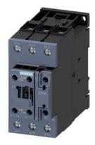
power contactor, AC-3e/AC-3, 41 A, 18.5 kW / 400 V, 3-pole, 24 V DC, 0.8-1.2\* Us, with integrated varistor, auxiliary contacts: 1 NO + 1 NC, screw terminal, size: S2, suitable for PLC outputs
