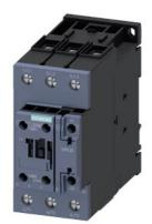
power contactor, AC-3e/AC-3, 41 A, 18.5 kW / 400 V, 3-pole, 24 V DC, 0.8-1.2\* Us, with integrated varistor, auxiliary contacts: 1 NO + 1 NC, screw terminal, size: S2, suitable for PLC outputs, upright mounting position
