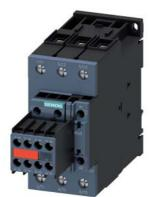
power contactor, AC-3e/AC-3, 41 A, 18.5 kW / 400 V, 3-pole, 230 V AC, 50/60 Hz, with plugged-in varistor, auxiliary contacts: 2 NO + 2 NC, screw terminal, size: S2, captive auxiliary switch
