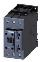
power contactor, AC-3e/AC-3, 41 A, 18.5 kW / 400 V, 3-pole, 480 V AC, 60 Hz, auxiliary contacts: 1 NO + 1 NC, screw terminal, size: S2  $\,$
