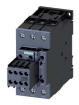
power contactor, AC-3e/AC-3, 41 A, 18.5 kW / 400 V, 3-pole, 230 V AC, 50 Hz, auxiliary contacts: 2 NO + 2 NC, screw terminal, size: S2, removable auxiliary switch
