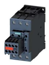
power contactor, AC-3e/AC-3, 41 A, 18.5 kW / 400 V, 3-pole, 230 V AC, 50 Hz, auxiliary contacts: 2 NO + 2 NC, screw terminal, size: S2, captive auxiliary switch
