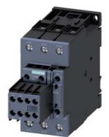
power contactor, AC-3e/AC-3, 41 A, 18.5 kW / 400 V, 3-pole, 220 V AC, 50/60 Hz, auxiliary contacts: 2 NO + 2 NC, screw terminal, size: S2, removable auxiliary switch
