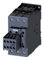
power contactor, AC-3e/AC-3, 41 A, 18.5 kW / 400 V, 3-pole, 110 V AC, 50 Hz / 120 V, 60 Hz, auxiliary contacts: 2 NO + 2 NC, screw terminal, size: S2, removable auxiliary switch
