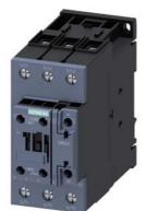
power contactor, AC-3e/AC-3, 41 A, 18.5 kW / 400 V, 3-pole, 110 V AC, 50 Hz / 120 V, 60 Hz, auxiliary contacts: 1 NO + 1 NC, screw terminal, size: S2
