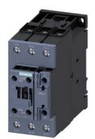
power contactor, AC-3e/AC-3, 41 A, 18.5 kW / 400 V, 3-pole, 110 V AC, 50 Hz / 120 V, 60 Hz, auxiliary contacts: 1 NO + 1 NC, screw terminal, size: S2, upright mounting position
