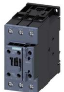
power contactor, AC-3e/AC-3, 41 A, 18.5 kW / 400 V, 3-pole, 48 V AC, 50 Hz, auxiliary contacts: 1 NO + 1 NC, screw terminal, size: S2  $\,$
