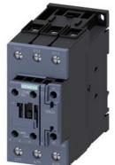
power contactor, AC-3e/AC-3, 41 A, 18.5 kW / 400 V, 3-pole, 110 V AC, 50/60 Hz, auxiliary contacts: 1 NO + 1 NC, screw terminal, size: S2  $\,$
