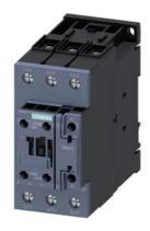
power contactor, AC-3e/AC-3, 41 A, 18.5 kW / 400 V, 3-pole, 24 V AC, 50 Hz, auxiliary contacts: 1 NO + 1 NC, screw terminal, size: S2, upright mounting position
