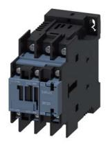
traction contactor, AC-3e/AC-3, 38 A, 18.5 kW / 400 V, 3-pole, 24 V DC, 0.7-1.25\* Us, electronic drive, with integrated varistor, auxiliary contacts: 1 NO + 1 NC, ring cable lug connection, size: S0
