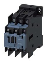
power contactor, AC-3e/AC-3, 38 A, 18.5 kW / 400 V, 3-pole, 125 V DC, auxiliary contacts: 1 NO + 1 NC, ring cable lug connection, size: S0  $\,$
