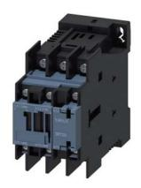
power contactor, AC-3e/AC-3, 38 A, 18.5 kW / 400 V, 3-pole, 24 V DC, auxiliary contacts: 1 NO + 1 NC, ring cable lug connection, size: S0  $\,$
