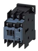
power contactor, AC-3e/AC-3, 38 A, 18.5 kW / 400 V, 3-pole, 220 V AC, 50 Hz / 240 V, 60 Hz, auxiliary contacts: 1 NO + 1 NC, ring cable lug connection, size: S0
