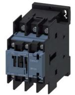
power contactor, AC-3e/AC-3, 38 A, 18.5 kW / 400 V, 3-pole, 100 V AC, 50 Hz / 100-110 V, 60 Hz, auxiliary contacts: 1 NO + 1 NC, ring cable lug connection, size: S0
