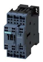
traction contactor, AC-3e/AC-3, 38 A, 18.5 kW / 400 V, 3-pole, 125 V DC, 0.7-1.25\* Us, electronic drive, with integrated varistor, auxiliary contacts: 1 NO + 1 NC, spring-loaded terminal, size: S0
