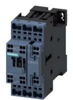
power contactor, AC-3e/AC-3, 38 A, 18.5 kW / 400 V, 3-pole, 21-28 V AC/DC, 50/60 Hz, with integrated varistor, auxiliary contacts: 1 NO + 1 NC, spring-loaded terminal, size: S0
