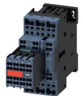
power contactor, AC-3e/AC-3, 38 A, 18.5 kW / 400 V, 3-pole, 230 V AC, 50/60 Hz, with plugged-in varistor, auxiliary contacts: 2 NO + 2 NC, spring-loaded terminal, size: S0, captive auxiliary switch
