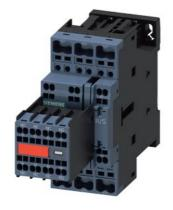
power contactor, AC-3e/AC-3, 38 A, 18.5 kW / 400 V, 3-pole, 230 V AC, 50/60 Hz, auxiliary contacts: 2 NO + 2 NC, spring-loaded terminal, size: S0, captive auxiliary switch, no surge suppressor retrofittable
