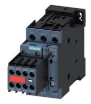
power contactor, AC-3e/AC-3, 38 A, 18.5 kW / 400 V, 3-pole, 24 V DC, with plugged-in diode combination, auxiliary contacts: 2 NO + 2 NC, screw terminal, size: S0, captive auxiliary switch
