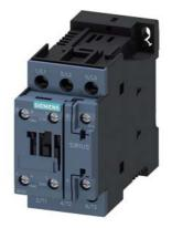
power contactor, AC-3e/AC-3, 38 A, 18.5 kW / 400 V, 3-pole, 220 V DC, auxiliary contacts: 1 NO + 1 NC, screw terminal, size: S0, India 40 A, Tu max. 50  $^{\circ}$ C
