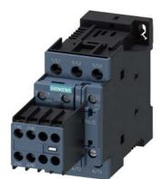
power contactor, AC-3e/AC-3, 38 A, 18.5 kW / 400 V, 3-pole, 24 V DC, auxiliary contacts: 2 NO + 2 NC, screw terminal, size: S0, removable auxiliary switch
