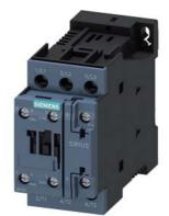
power contactor, AC-3e/AC-3, 38 A, 18.5 kW / 400 V, 3-pole, 24 V DC, auxiliary contacts: 1 NO + 1 NC, screw terminal, size: S0, upright mounting position
