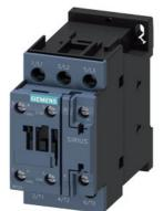
power contactor, AC-3e/AC-3, 38 A, 18.5 kW / 400 V, 3-pole, 220 V AC, 50 Hz / 240 V, 60 Hz, auxiliary contacts: 1 NO + 1 NC, screw terminal, size: S0
