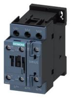
power contactor, AC-3e/AC-3, 38 A, 18.5 kW / 400 V, 3-pole, 230 V AC, 50 Hz, auxiliary contacts: 1 NO + 1 NC, screw terminal, size: S0, upright mounting position
