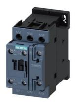
power contactor, AC-3e/AC-3, 38 A, 18.5 kW / 400 V, 3-pole, 110 V AC, 50 Hz / 120 V, 60 Hz, auxiliary contacts: 1 NO + 1 NC, screw terminal, size: S0
