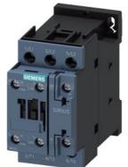
power contactor, AC-3e/AC-3, 38 A, 18.5 kW / 400 V, 3-pole, 110 V AC, 50 Hz, auxiliary contacts: 1 NO + 1 NC, screw terminal, size: S0
