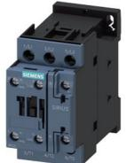
power contactor, AC-3e/AC-3, 38 A, 18.5 kW / 400 V, 3-pole, 24 V AC, 50/60 Hz, auxiliary contacts: 1 NO + 1 NC, screw terminal, size: S0
