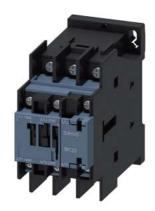
power contactor, AC-3e/AC-3, 32 A, 15 kW / 400 V, 3-pole, 24 V AC, 50/60 Hz, auxiliary contacts: 1 NO + 1 NC, ring cable lug connection, size: S0  $\,$
