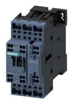
power contactor, AC-3e/AC-3, 32 A, 15 kW / 400 V, 3-pole, 21-28 V AC/DC, 50/60 Hz, with integrated varistor, auxiliary contacts: 1 NO + 1 NC, spring-loaded terminal, size: S0
