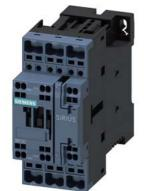
power contactor, AC-3e/AC-3, 32 A, 15 kW / 400 V, 3-pole, 24 V DC, auxiliary contacts: 1 NO + 1 NC, spring-loaded terminal, size: S0
