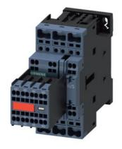
power contactor, AC-3e/AC-3, 32 A, 15 kW / 400 V, 3-pole, 110 V AC, 50 Hz / 120 V, 60 Hz, auxiliary contacts: 2 NO + 2 NC, spring-loaded terminal, size: S0, captive auxiliary switch, no surge suppressor retrofittable
