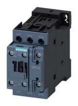
power contactor, AC-3e/AC-3, 32 A, 15 kW / 400 V, 3-pole, 24 V DC, auxiliary contacts: 1 NO + 1 NC, screw terminal, size: S0, upright mounting position
