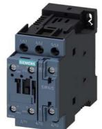
power contactor, AC-3e/AC-3, 32 A, 15 kW / 400 V, 3-pole, 24 V DC, auxiliary contacts: 1 NO + 1 NC, screw terminal, size: S0, communication-capable
