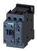
power contactor, AC-3e/AC-3, 32 A, 15 kW / 400 V, 3-pole, 277 V AC, 60 Hz, auxiliary contacts: 1 NO + 1 NC, screw terminal, size: S0  $\,$
