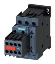
power contactor, AC-3e/AC-3, 32 A, 15 kW / 400 V, 3-pole, 230 V AC, 50/60 Hz, auxiliary contacts: 2 NO + 2 NC, screw terminal, size: S0, captive auxiliary switch, no surge suppressor retrofittable
