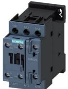
power contactor, AC-3e/AC-3, 32 A, 15 kW / 400 V, 3-pole, 110 V AC, 50 Hz / 120 V, 60 Hz, auxiliary contacts: 1 NO + 1 NC, screw terminal, size: S0
