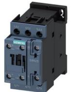
power contactor, AC-3e/AC-3, 32 A, 15 kW / 400 V, 3-pole, 110 V AC, 50/60 Hz, auxiliary contacts: 1 NO + 1 NC, screw terminal, size: S0
