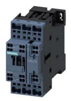
power contactor, AC-3e/AC-3, 25 A, 11 kW / 400 V, 3-pole, 95-130 V AC/DC, 50/60 Hz, with integrated varistor, auxiliary contacts: 1 NO + 1 NC, spring-loaded terminal, size: S0
