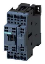
power contactor, AC-3e/AC-3, 25 A, 11 kW / 400 V, 3-pole, 21-28 V AC/DC, 50/60 Hz, with integrated varistor, auxiliary contacts: 1 NO + 1 NC, spring-loaded terminal, size: S0
