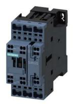
power contactor, AC-3e/AC-3, 25 A, 11 kW / 400 V, 3-pole, 24 V DC, with plugged-in diode combination, auxiliary contacts: 1 NO + 1 NC, spring-loaded terminal, size: S0
