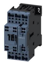
power contactor, AC-3e/AC-3, 25 A, 11 kW / 400 V, 3-pole, 110 V AC, 50 Hz / 120 V, 60 Hz, with plugged-in RC element, auxiliary contacts: 1 NO + 1 NC, spring-loaded terminal, size: S0
