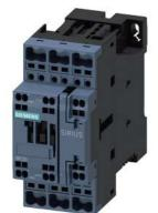
power contactor, AC-3e/AC-3, 25 A, 11 kW / 400 V, 3-pole, 24 V DC, auxiliary contacts: 1 NO + 1 NC, spring-loaded terminal, size: S0
