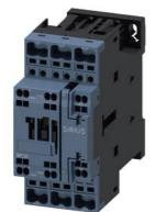
power contactor, AC-3e/AC-3, 25 A, 11 kW / 400 V, 3-pole, 400 V AC, 50 Hz, auxiliary contacts: 1 NO + 1 NC, spring-loaded terminal, size: S0  $\,$
